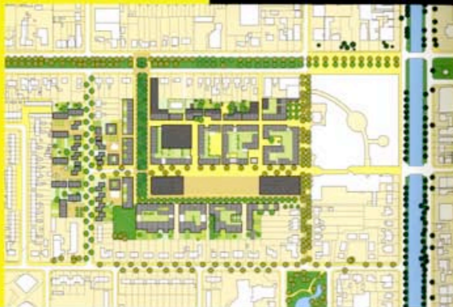
• New Town Centre, Groningen, 2002 : urban development plan for a 400-hectare site, with 480 housing units and 22,500 square metres of retail and commercial spaces, Netherlands, 2002-04 (left) site plan showing new alternatives emerging from a traditional type
